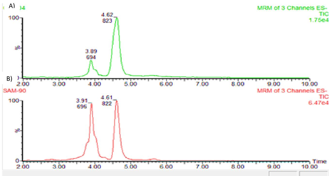
**Fig. (1):** Multiple reaction monitoring (MRM) chromatograms obtained for chromatographic separation of galactitol and galactose-1-phosphate (G-1-P). A) Control RBC sample supplemented with 12.5  $\mu$ M of G-1-P and 6  $\mu$ M of galactitol. B) Galactosemia patient sample containing 306  $\mu$ M (8 mg/dl) G-1-P and 4  $\mu$ M galactitol. Retention times: 3.9 min for G-1-P and 4.6 min for galactitol.
